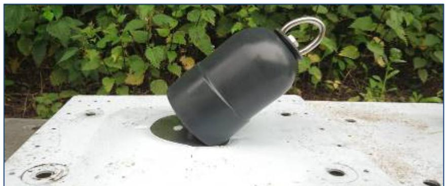
The image here shows the post after a 200kg load was arrested, and a subsequent applied 13kN load for 3 minutes was held as per the requirements of the tests.
