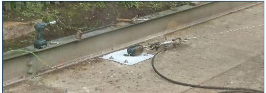
It can be seen in this image that the post has completely tipped and that the base plate has deformed. The connecting assembly inside the post can also be seen to be bent over.
