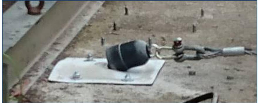
It can be seen that the post has tipped over, is bent and the leading edge is compressed against the base plate.
